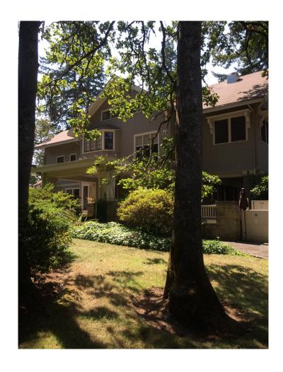
Historic Materials: Tenino stone-cut block foundation, columns, facade, and porte-cochere; painted wood columns, corbels, eave brackets, and shingles; most likely the original 6/1 double-hung sash windows.
