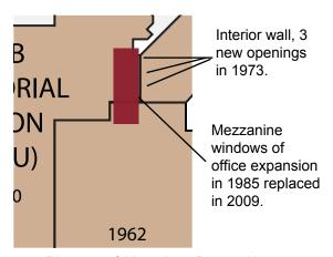
Diagram of Alterations Due to 1973 Southeast Attachment
