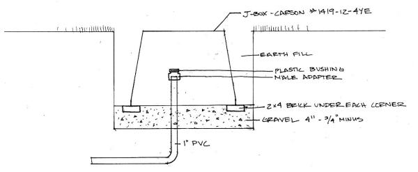
• Plan view detail of Mow slab for pole light base in lawn conditions adjacent to sidewalks:
