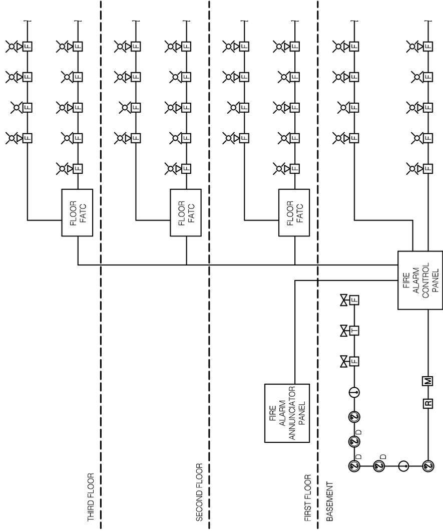
**FIRE ALARM SYSTEM RISER DIAGRAM**
