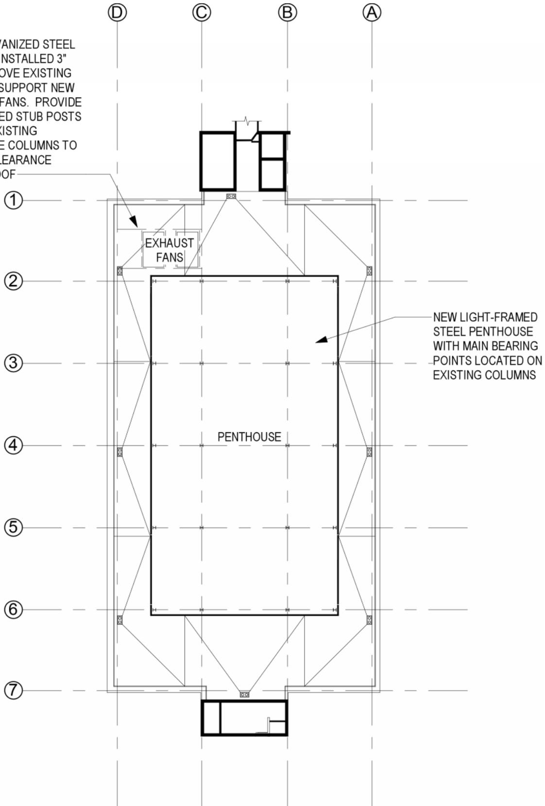
NEW LIGHT-FRAMED STEEL PENTHOUSE WITH MAIN BEARING POINTS LOCATED ON EXISTING COLUMNS
