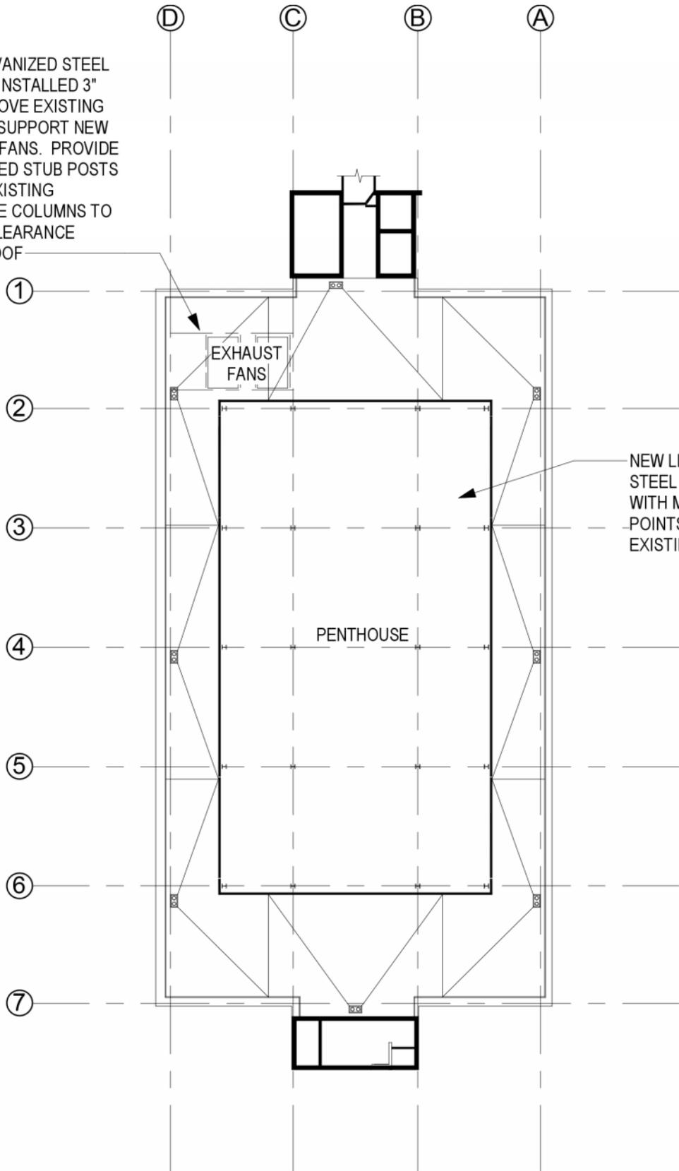
NEW LIGHT-FRAMED STEEL PENTHOUSE WITH MAIN BEARING POINTS LOCATED ON EXISTING COLUMNS
