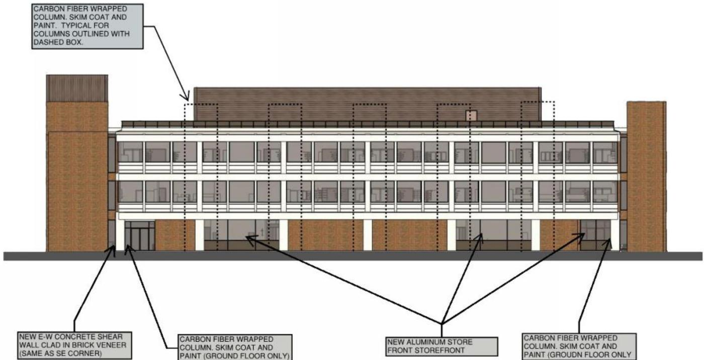
**EAST ELEVATION (WEST ELEVATION SIMILAR)**
