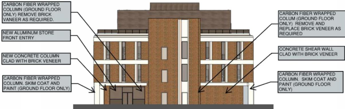
**SOUTH ELEVATION (NORTH ELEVATION SIMILAR)**
