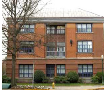
Composition - Buildings should be vertically composed of three parts: top, middle, and bottom. Provide distinction through the use of horizontal lines, such as banding, use of different materials, or variation in patterns and textures.
