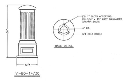
b. Permanent Bollards, OFCI: VISCO #VI-BO-14, powder-coated UO Green.
