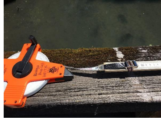
Figure 2 The meter stick-measuring tape combination tool
