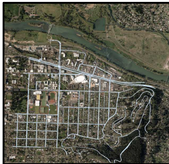
Fig. 8 and Fig. 9 – Calculation of stormwater entering the Millrace. The total area of streets diverting storm water into the Millrace is 3,510,358 square feet, which is 0.126 square miles. Averaging the highest and lowest rainfall years, the Millrace is subjected to City street storm water runoff equal to about 105 million gallons.
